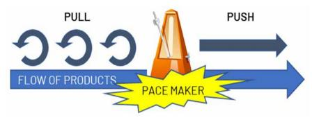
The pace of production, Takt time, is the time required to produce a single component or an entire product in order to meet and not exceed customer demand.
